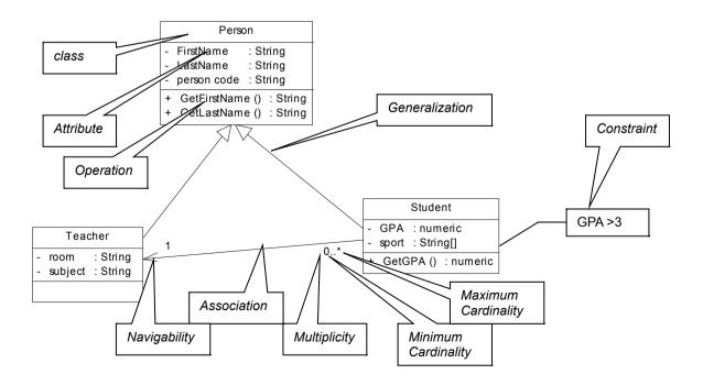
In the essential part of a class diagram as it is shown in picture are listed:
